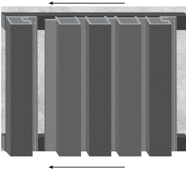
The second Panel can now be slotted next to the first using the tongue and groove method. The non-grooved lip of the second panel will conceal the screws from the first and secured on the top grooved lip. Repeat this process with each Slatted Panel until you reach the required coverage, making sure that each Panel is securely fixed to the Batten underneath.
