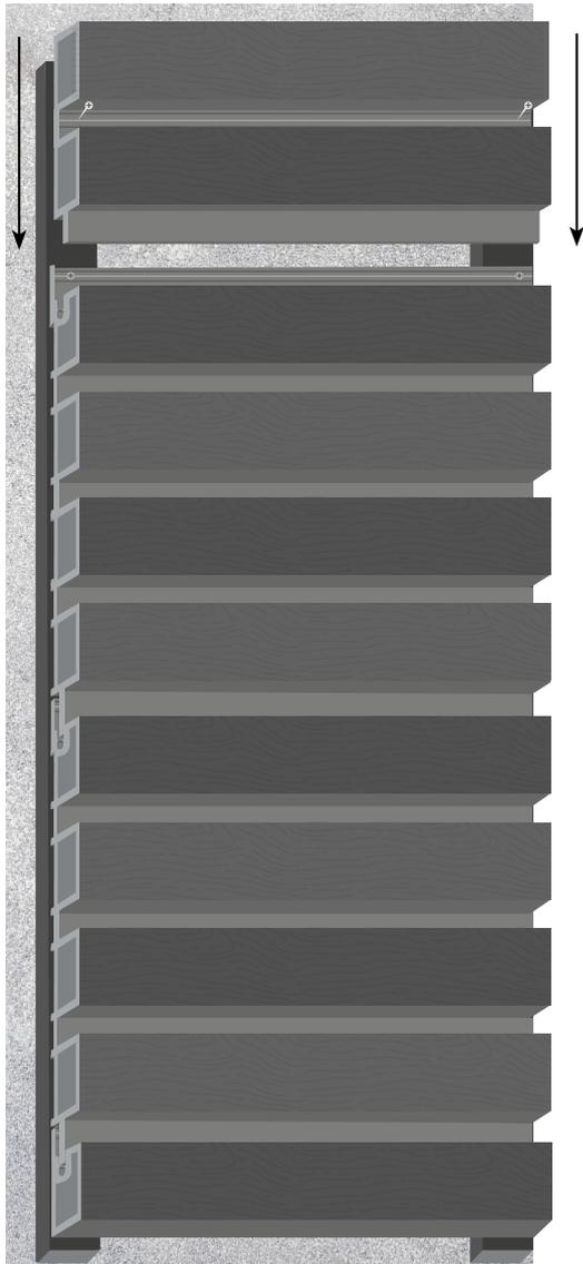
The second Panel can now be slotted on top of the first using the tongue and groove method. The non-grooved lip of the second panel will conceal the screws from the first and secured on the top grooved lip. Repeat this process with each Slatted Panel until you reach the required height and coverage, making sure that each panel is securely fixed to the Batten underneath.
