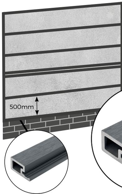
Before the Slatted Cladding Panels can be installed, the Single Start Profile Trims must be fixed in place alongside the Battens before any of the Panels can be installed using 20mm screws. A 5mm expansion gap should be left between the Slatted Panels and the Internal/ External Corner and Double End Profile Trim. It is recommended that each section is fully installed at a time for consistency.
