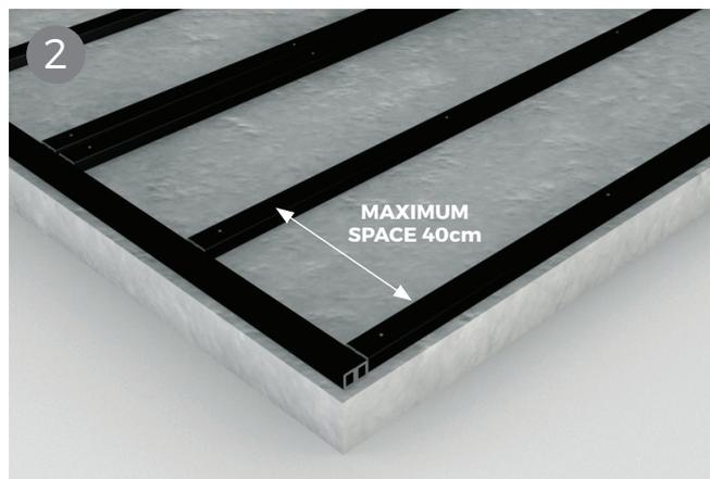
Step 2, The maximum recommended space between joist rows depends on the angle at which you intend to lay your boards in relation to the joists, but should **never exceed 400mm**, please see diagram (above).
